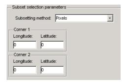
**Tile.** In HDF-EOS Grid data, a rectilinear grid overlays a map. Each rectangle defined by the horizontal and vertical lines of the grid is referred to as a tile. If the HDF-EOS Grid data is stored as tiles, you can import a subset of the data by specifying the coordinates of the tile you are interested in. Tile coordinates are 1-based, with the upper-left corner of a two-dimensional data set identified as 1,1. In a three-dimensional data set, this tile would be referenced as 1,1,1.
