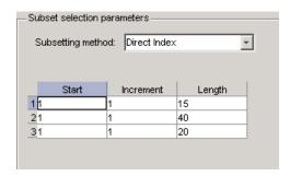
Each row represents a dimension in the data set and each column represents these subsetting parameters:
