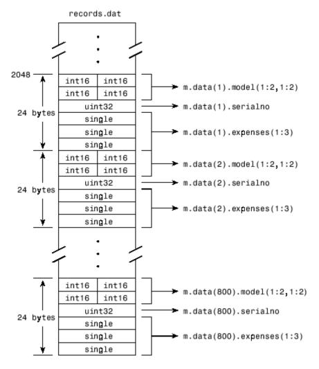
The figure below shows the ordering of the array elements more closely. In particular, it illustrates that MATLAB arrays are stored on the disk in column-major order. The sequence of array elements in the mapped file is row 1, column 1; row 2, column 1; row 1, column 2; and row 2, column 2.
