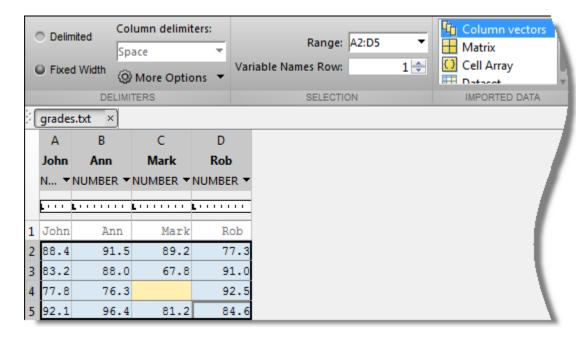
The Import Tool recognizes that grades.txt is a fixed width file. In the Imported Data section, select how you want the data to be imported, for instance, as column vectors or as a single matrix.
