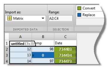
Select the data range and the type of variable to create (matrix, column vectors, or cell array). For example, the data in the previous figure corresponds to a 3-by-3 matrix named untitled. You can edit the variable
