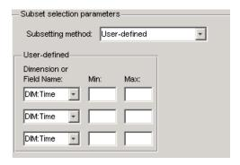
When specifying user-defined parameters, you must first specify whether you are subsetting along a dimension or by field. Select the dimension or field by name using the **Dimension or Field Name** menu. Dimension names are prefixed with the characters DIM:.
