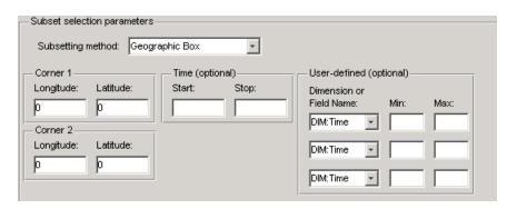
Optionally, you can further define the subset of data you are interested in by using Time parameters (see "Time" on page 6-64) or by specifying other User-Defined subsetting parameters (see "User-Defined" on page 6-65).
